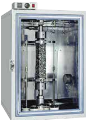
Direct tension / compression test Uniaxial low temperature tension test Thermal Stress Restrain Specimen test
