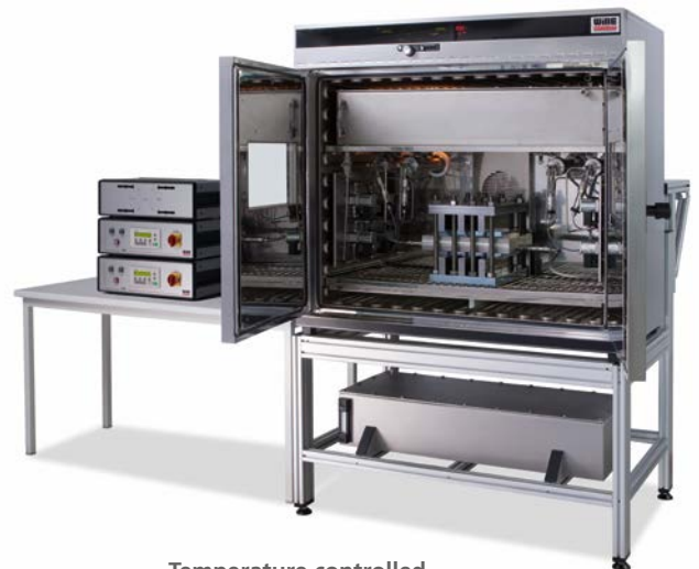
Temperature controlled permeability testing system
