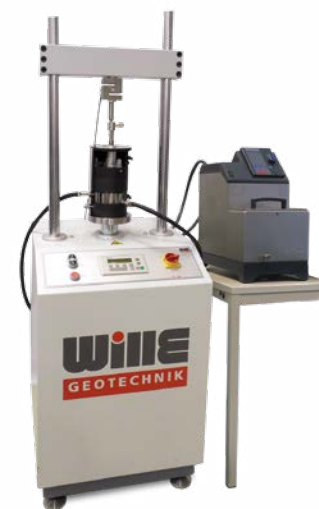
Thermal consolidation testing system (THM)
