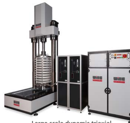
Large scale dynamic triaxial testing systems
