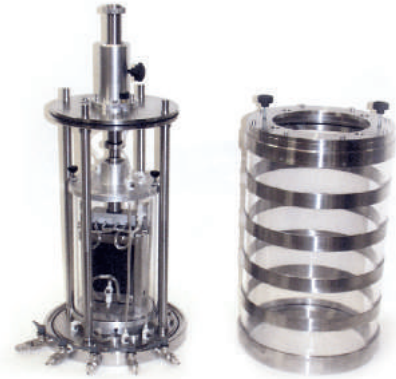
Double wall biaxial cell for plane strain tests with unsaturated conditions.
