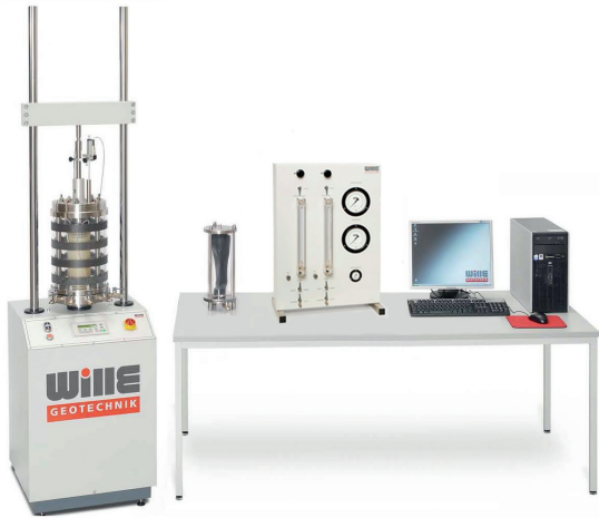
Conventional and unsaturated triaxial testing system
