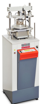
Consolidation test system
