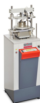
Uniaxial compression test
