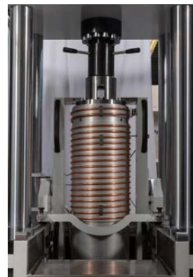
High pressure/ high temperature triaxial cell with external cooling system
