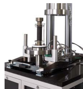
High pressure / high temperature triaxial cell with sample adapter (internal view)
