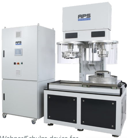
Wehner/Schulze device for determination of friction after polishing
